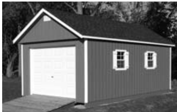
12x20' Garage, 7/12 roof pitch
